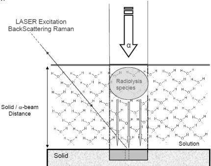
Figure 1: *In situ* Raman spectroscopic device experiment under  ${}^{4}\text{He}^{2+}$  ions beam irradiation onto the ARRONAX facility vertical beam line (Borosilicate Glass Disc Thickness =  $150 \pm 10 \, \mu\text{m}$ , Electrolyte Thickness =  $5 \, \text{mm}$ )
