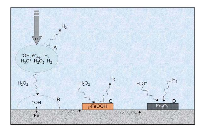
Figure 5: Scheme of iron corrosion mechanisms under  ${}^4\text{He}^{2+}$  ions irradiation, (A) water radiolysis, (B)  $H_2O_2$  catalytic decomposition and iron oxidation, (C) Lepidocrocite  $\gamma$ -FeOOH formation with  $H_2$  production (carbon steel sample), (D) Magnetite Fe<sub>3</sub>O<sub>4</sub> formation with  $H_2$  consumption (pure iron sample)
