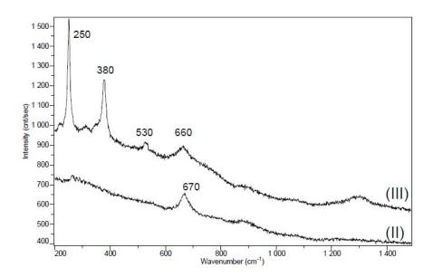
Figure 2: Corroded iron sample (set II) with Raman band of magnetite phase at 670 cm<sup>-1</sup> and corroded carbon steel sample (set III) with Raman bands of lepidocrocite phase at 250/380/530/660 cm<sup>-1</sup> identified in the literature [48]
