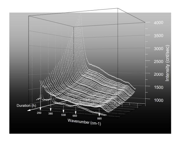
Figure 4: Raman spectra of set IV during the *in situ* experiment with an experimental time of 15 h after the irradiation. Corroded carbon steel sample with formation vs. time of the typical Raman bands of lepidocrocite phase at 250/380/530/660 cm<sup>-1</sup> and  $H_2O_2$  Raman band at 885 cm<sup>-1</sup>
