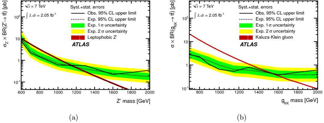
Figure 4: Observed (black points) and expected (dashed line) upper limits on  $\sigma \times BR(Z' \rightarrow t\bar{t})$  (a) and  $\sigma \times BR(g_{KK} \rightarrow t\bar{t})$  for the lepton plus jets boosted channel. The dark and light green bands show the range in which the limit is expected to lie in 68% and 95% of experiments, respectively <sup>4</sup>.
