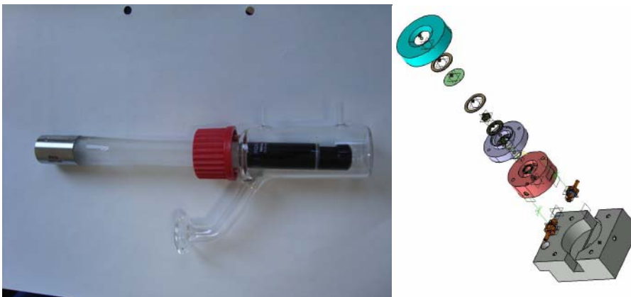
Figure 5: Left: New measurement cell with UV-VIS probe, Right: Schematic picture of the new In situ Raman spectroscopic cell
