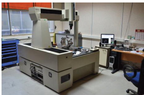
Figure 2: Picture of Mitutoyo 3D machine (precision and resolution of 5/1\mu\text{m} ) used for dimensional testing, with the chamber body and special BPM positioning tool at the edge.
