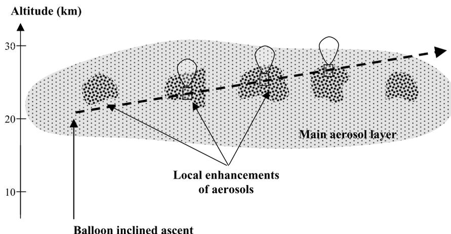
**Figure 2.** Geometry of measurements during some ascents of the stratospheric balloons. The presence of local enhancements around 25 km crossed obliquely during the slant ascent of the gondola (represented by the dashed line) can produce three consecutive artificial thin layers on the STAC profiles.
