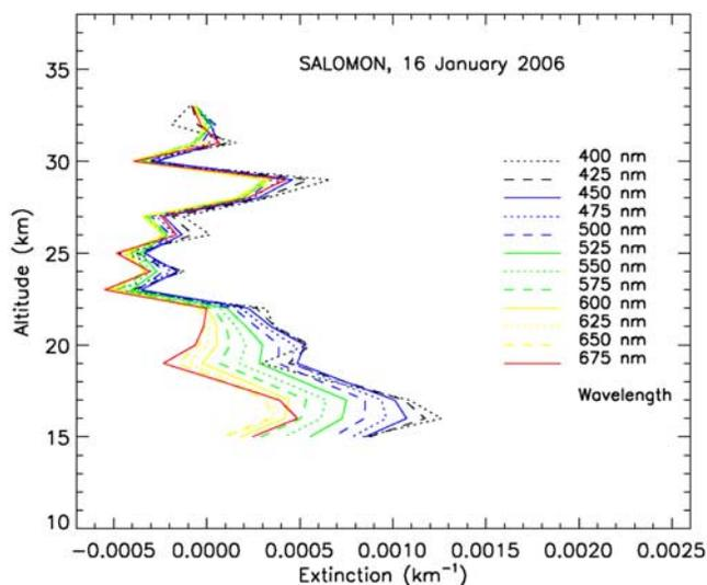
**Figure 3.** Wavelength dependence of aerosol extinction measured by SALOMON on 16 January 2006 inside the northern polar vortex. For clarity, the error bars (about  $1 \times 10^{-4}$  at each wavelength) are omitted. The negative values above 22 km can appear during the spatial inversion if the contribution of aerosols is not equal to zero in the reference spectrum and/or if local enhancements are present around the float altitude.
