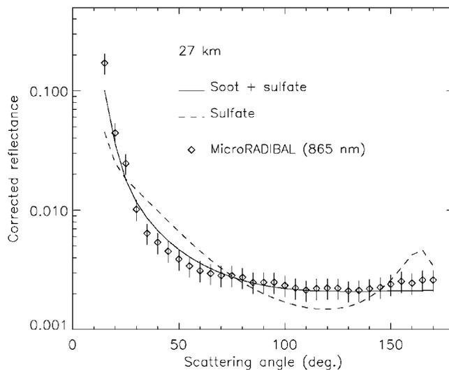
**Figure 9.** Comparison between MicroRADIBAL corrected reflectance at 27 km and two diagrams computed for bimodal size distributions: (1) with a mode of soot (see Figure 8) and a mode of sulfate particles and (2) with two modes of sulfate particles. The MicroRADIBAL errors are about 10%.
