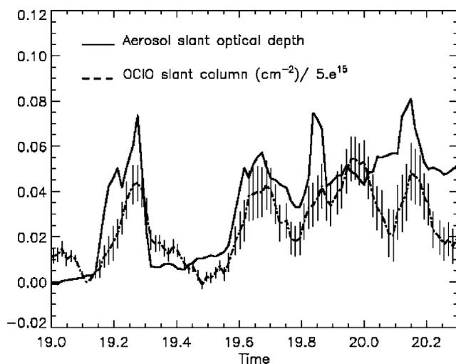
**Figure 5.** Comparison between aerosol slant optical depths averaged in the 400- to 675-nm range and the OCIO slant column above the gondola altitude, obtained by SALOMON on 16 January 2006.
