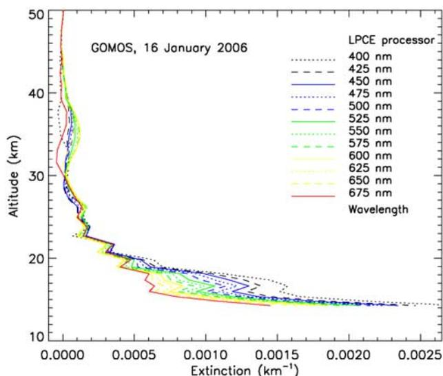
**Figure 6.** Wavelength dependence of aerosol extinction measured by GOMOS obtained with the “LPCE processor”, for 16 January 2006 inside the northern polar vortex. For clarity, the error bars (about  $1 \times 10^{-4} \text{ km}^{-1}$  at each wavelength) are omitted.
