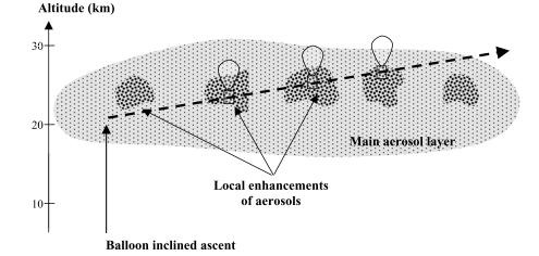
**Figure 2.** Geometry of measurements during some ascents of the stratospheric balloons. The presence of local enhancements around 25 km crossed obliquely during the slant ascent of the gondola (represented by the dashed line) can produce three consecutive artificial thin layers on the STAC profiles.
