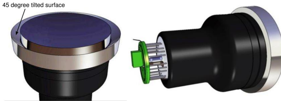
Figure 2. A drawing of the expansion cone mounted on a PMT.
