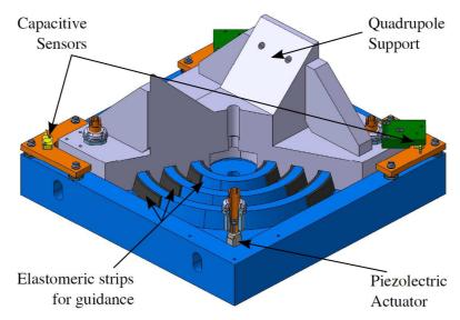
Figure 4. 3D view with the quadrupole support.
