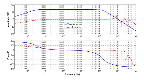
*Figure 6. Velocity sensor and accelerometer transfer functions.*
