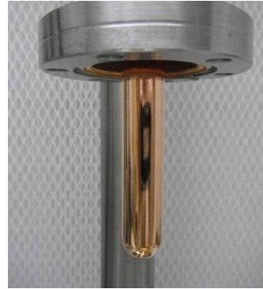
Figure 6: Electropolished antenna tip.
