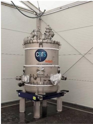
Figure 5: The first cryomodule in GANIL, ready for installation in the linac tunnel.
