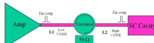
Figure 7: Power chain of the SC linac cavities.
