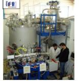
Figure 3: The SPIRAL2 superconducting cryomodules (left:  $\beta_0$ =0.07 – 1 cavity, right:  $\beta_0$ =0.12 – 2 cavities).
