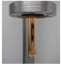
Figure 6: Electropolished antenna tip.
