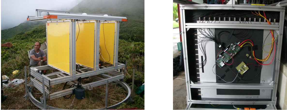
Figure 1. Left : Picture of a muon telescope in horizontal position. The three detection planes are protected by the yellow frames. Right : The inner part of a matrix : active XY scintillator planes, PMT and readout electronics.
