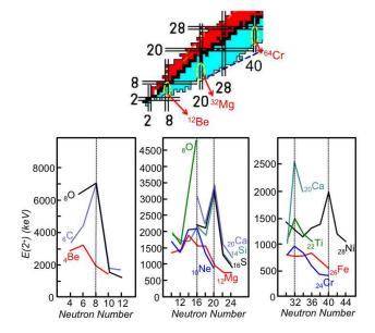
FIG. 1: Top: The parts of the chart of the nuclides in which the same mechanisms leading to the islands of inversion occurs are indicated by yellow dashed ellipsoids. Bottom: Evolution of the  $2_1^+$  energies in the N=8 (Be, C, O), 20 (O, Ne, Mg, Si, S and Ca) and 40 (Ni, Fe, Cr, Ti, Ca) regions. The rise in  $2_1^+$  energies at N=8, 20 and 40 no longer exists for neutronrich nuclei. Rather rises in  $2_1^+$  energies appear at N=16 and N=32.
