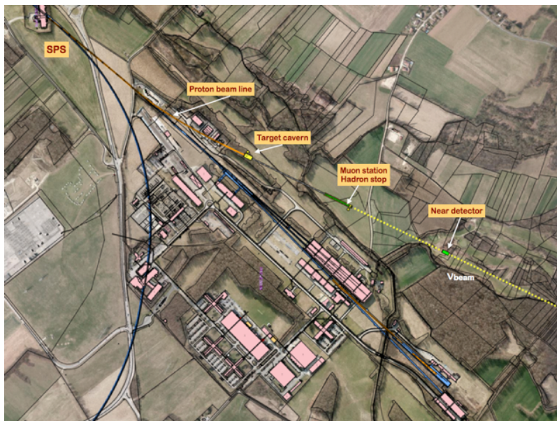
Figure 3: The baseline layout for the LBNO neutrino facility in the vicinity of the CERN North Area.
