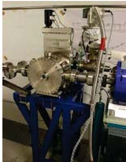
Figure 4: Smith-Purcell apparatus installed in the SOLEIL injector linac.
