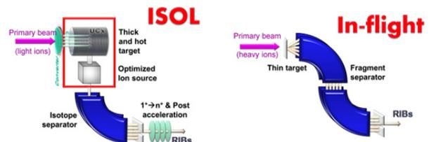
Figure 1: ISOL and In-flight RIB production methods.
