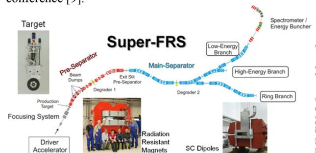
Figure 3 : FAIR Super-FRS with its three exit branches.
