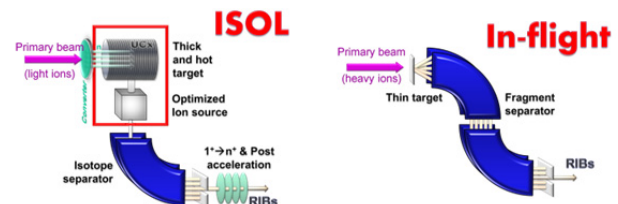
Figure 1: ISOL and In-flight RIB production methods.
