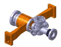
Figure 3: Drawing of the 2998MHz ThomX electron gun.
