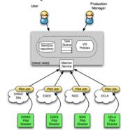
Figure 1: DIRAC computing structure.
