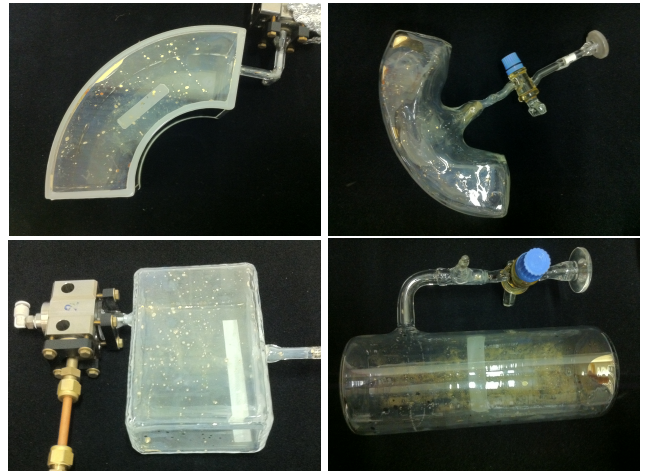
Figure 1. Examples of cells used as polarized helium 3 containers.
