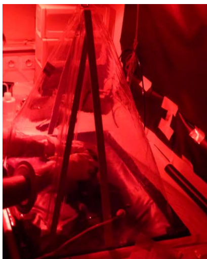
Figure 1: a portable glow bag for the sample manipulation.
