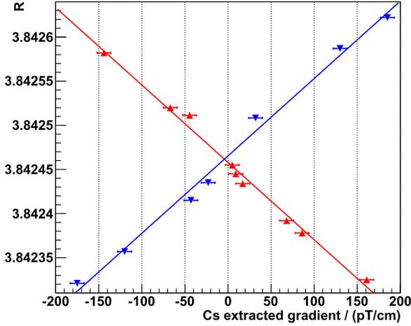
**Fig. 3.** Neutron to mercury frequency  $R = f_n/f_{\text{Hg}}$  plotted as a function of the field gradient. Upwards-pointing (red) and downwards-pointing (blue) triangles represents runs in which  $B_0$  was pointing upwards and downwards, respectively. The vertical error bars are smaller than the size of the triangles.
