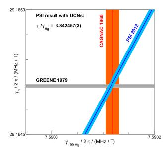
**Fig. 4.** 1-sigma allowed regions in the  $\gamma_n$ ,  $\gamma_{Hg}$  plane. Our final value for the neutron to mercury magnetic moment ratio (18) here labeled as "PSI 2012" forms the diagonal band. The horizontal band is the neutron magnetic moment (1) value from Greene et al. and the vertical band is from the measurement of the mercury magnetic moment (2) by Cagnac.
