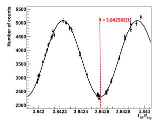
Fig. 2. Ramsey fit for the run 6043. In this run the goodness-of-fit is quantified by  $\chi^2/d.o.f.=1.3.$
