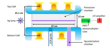
**Fig. 1.** Vertical cut through the inner part of the nEDM apparatus. Schematically indicated are the precession chamber, the mercury comagnetometer and the Cs magnetometer array.
