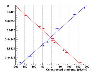
**Fig. 3.** Neutron to mercury frequency  $R = f_n/f_{Hg}$  plotted as a function of the field gradient. Upwards-pointing (red) and downwards-pointing (blue) triangles represents runs in which  $B_0$  was pointing upwards and downwards, respectively. The vertical error bars are smaller than the size of the triangles.
