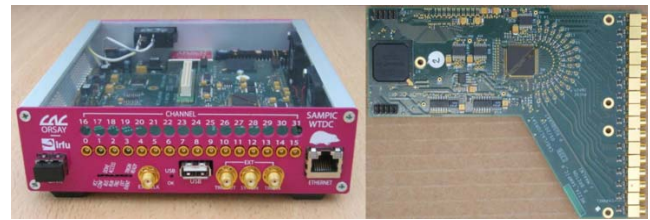
Fig. 9: SAMPIC acquisition module (left) and mezzanine (right).
