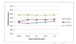
Figure 4: Measured FWHM bunch of <sup>36</sup>Ar<sup>+18</sup> versus beam intensity.
