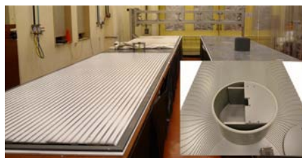
Figure 54: AMIGA scintillator detector, illustrating the assembly of a 10\text{ m}^2 module. Strips are grouped in two sets of 32 strips on each side of the electronics dome located at the center of the detector. The inset shows a detailed view of the manifold fiber routing and optical connector. The multi-anode PMT and front end electronics board are hosted in the central dome. Once deployed, access to the buried setup is provided by an inspection pipe.
