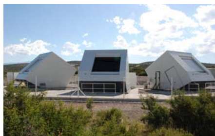
Figure 50: Photo of the three HEAT telescopes in tilted mode. The container for DAQ, slow control, and calibration hardware is behind the enclosure of the second telescope.
