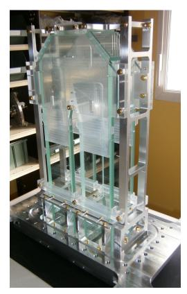
Figure 5. Bare float-glass structure held by the aluminium and PMMA support.
