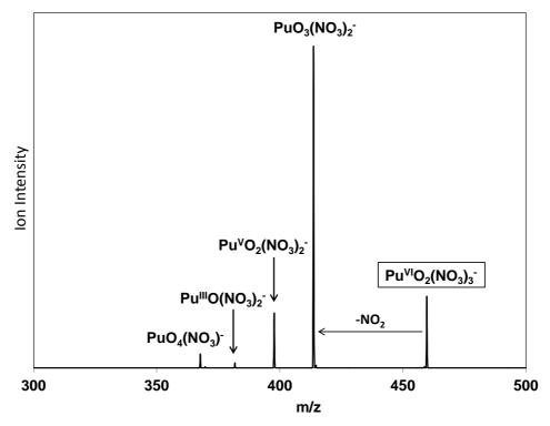
**Figure 3.** CID mass spectrum of  $PuO_2(NO_3)_3^-$ . The dominant channel is to produce  $PuO_3(NO_3)^-$ . Another significant channel is production of  $PuO_2(NO_3)_2$ .
