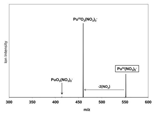
**Figure 2.**CID mass spectrum of  $Pu(NO_3)_5^-$ . The dominant channel is to produce plutonyl(VI) nitrate. A very small amount of  $PuO_3(NO_3)_2^-$  is also produced, presumably by loss of a third neutral NO<sub>2</sub> molecule from the dominant intermediate.
