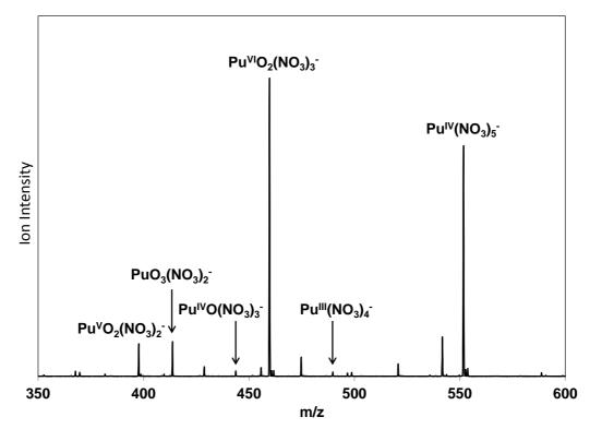
**Figure 1.**ESI mass spectrum of the plutonium nitrate solution. The assignments of the minor  $Pu(NO_3)_4^-$  and  $PuO(NO_3)_3^-$  peaks were confirmed from their CID spectra (Figs. S1 and S2). CID of  $Pu(NO_3)_5^-$  and  $PuO_2(NO_3)_3^-$  are discussed below.
