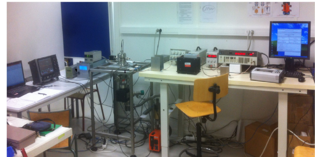
Figure 2: (a) Scheme and (b) View of the Coaxial resonator multipacting test bench.
