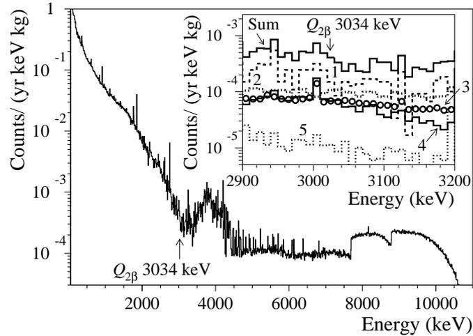
**FIGURE 2.** Energy spectra of 48  $\text{Zn}^{100}\text{MoO}_4$  detectors in EDELWEISS set-up simulated with the help of GEANT4 package. (Inset) The main components of background are shown: (1) surface contamination of  $\text{Zn}^{100}\text{MoO}_4$  crystals, (2) radioactive contamination of the reflecting foil surrounding the crystal, (3) bulk contamination of  $\text{Zn}^{100}\text{MoO}_4$  crystals, contamination of copper holders (4) and PTFE clamps (5).
