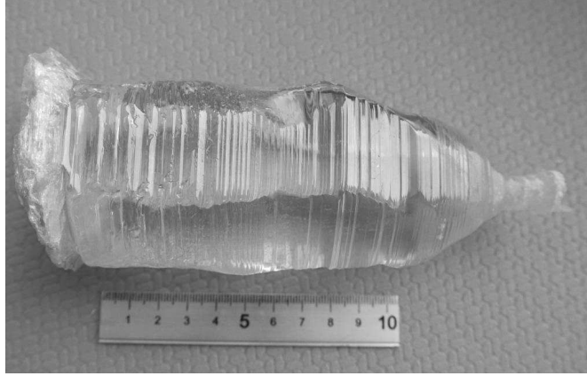
FIGURE 1. Boule of \text{Zn}^{100}\text{MoO}_4 crystal with mass \approx 1.4 kg produced from molybdenum isotopically enriched in ^{100}\text{Mo} .
