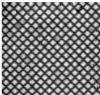
Fig. 8. X-ray resolution target image of the \text{Lu}_{1.56}\text{Gd}_{0.41}\text{Eu}_{0.03}\text{O}_3 crystal. The field view is 1.3 \times 1.3\ \text{mm}^2 and the grid lines thickness is \sim 25\ \mu\text{m} .
