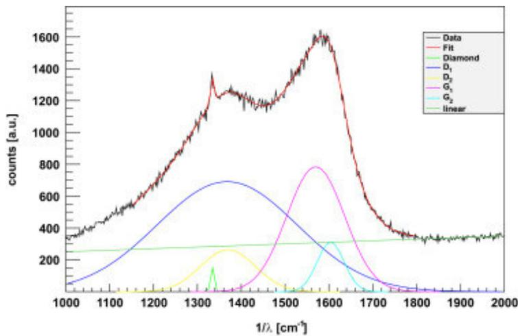
Fig. 4. Raman spectrum for the seed side of a channel grown at 60 mW and 2000  $\mu\text{m s}^{-1}$ . Individual contributions of the fitted functions are shown.
