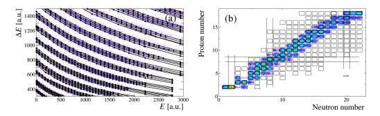
Fig. 8. Result of the automatic isotopic line extraction applied to a Si-Si matrix of FAZIA ( $\theta \sim 7^{\circ}$ ) in the Ar+Sn at 25 MeV/A reaction: (a) isotopic identification grid; (b) isotopic distribution after linearization.
