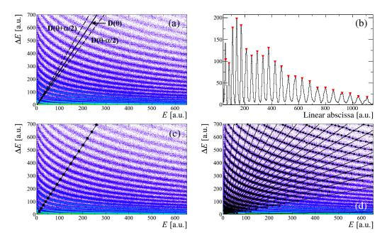
Fig. 1. Illustration of the different steps of the SPIDER Identification: (a) definition of the projection; (b) projection on line  $D(\theta)$  and localization of maxima; (c) positioning of the maxima on the  $\Delta E - E$  matrix; (d) weaving of the spiderweb.
