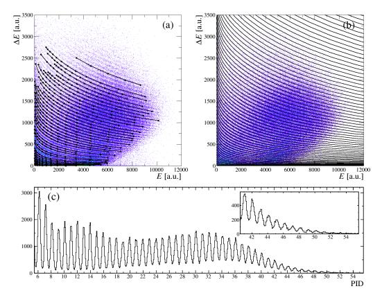
Fig. 6. Example of coupling between the SPIDER Identification method and a functional fit [14] on a Si-CsI(Tl) matrix of INDRA ( $\theta \sim 8.5^{\circ}$ ). Data come from the Ta+Zn at 39 MeV/A reaction measured at GANIL.
