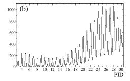
Fig. 5. Same as Fig. 2 for energy versus rise time of the charge signal in the first silicon layer matrix of FAZIA ( $\theta \sim 7^{\circ}$ ). Data come from the Kr+Sn at 35 MeV/A reaction measured at LNS [22,23].
