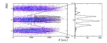
Fig. 7. Illustration of the isotopic identification method in PID-E matrices. Si-Si matrices (see Fig. 4).
