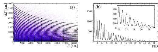
Fig. 2. Application of the SPIDER Identification method on a Si-CsI(Tl) matrix of INDRA ( $\theta \sim 17^{\circ}$ ). PID stands for particle identification obtained after linearization of the matrix with the identification grid. Data come from the Ta+Zn at 39 MeV/A reaction measured at GANIL.
