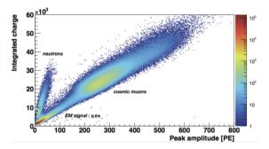
Fig. 3 EM / neutron /muon Discrimination, Integrated charge vs peak amplitude for signals collected by fiber-MMPC (1PE=80keV).
