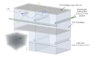
Fig. 2. IBD interaction in the detection elements and deposited energy due to an IBD event in the SoLid detector
