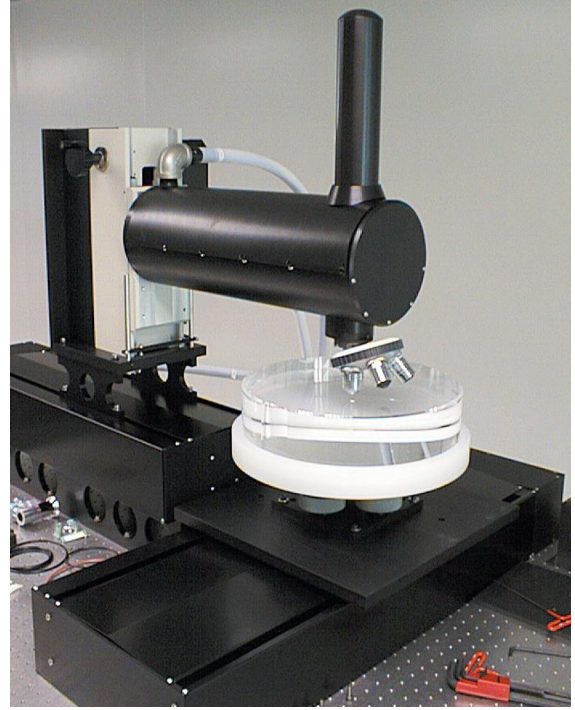
FIG. 1. Micromap optical profiler used for the measurement of the RoC of coated cantilever blades.
