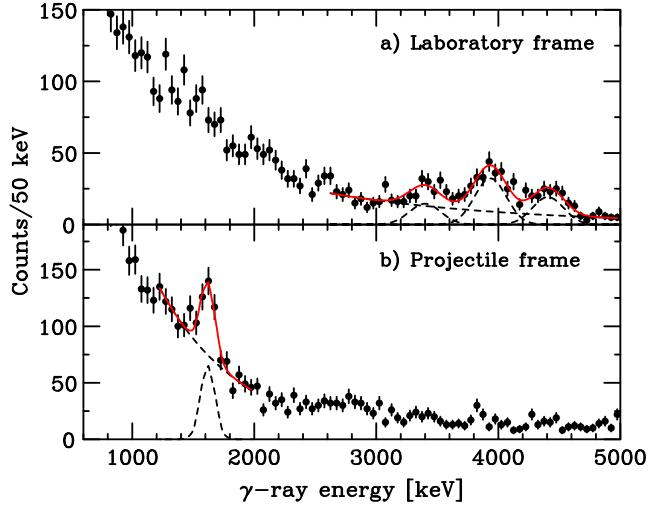
Fig. 2. (Color online.) The  $\gamma$ -ray energy spectrum in: a) the target frame, and b) the projectile frame, coincident with incoming  $^{20}\text{C}$  and outgoing  $^{20}\text{C}$  ions. In the target frame, the 4.4 MeV peak originates from the  $^{12}\text{C}(2_1^+)$  state (see text). The projectile frame peak at 1.6 MeV originates from the  $^{20}\text{C}(2_1^+)$  state.
