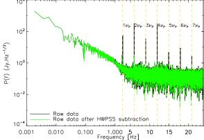
Fig. 4. TOI (*left*) and power spectrum (*right*) of an observation of Orion OMC-1 for a single KID. Raw data are presented in black and the Half Wave Plate systematic signal (HWPSS) subtracted data in green.
