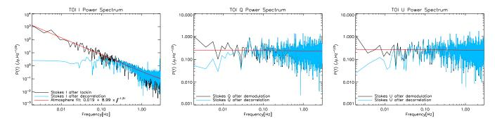
**Fig. 6.** From left to right: power spectra of the Stokes *I*, *Q*, and *U* pure TOIs (black) after applying the lock-in procedure to the raw data in Fig. 4. A bandpass filter ([0.01, 2.9] Hz) was applied to reject any high-frequency noise and half wave plate systematic signal (HWPSS) residual at the fourth harmonics. In blue we also show the power spectra after applying the decorrelation procedure to the demodulated data. See Sect. 4.4 for details.
