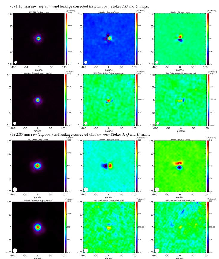
Fig. 7. Uranus Stokes I, Q and U maps in Nasmyth coordinates at 260 GHz **a**) and 150 GHz **b**) before and after leakage correction. After the leakage correction, we are left with a residual instrumental polarization below 1% (0.7% at 1.15 mm and 0.6% at 2.05 mm).
