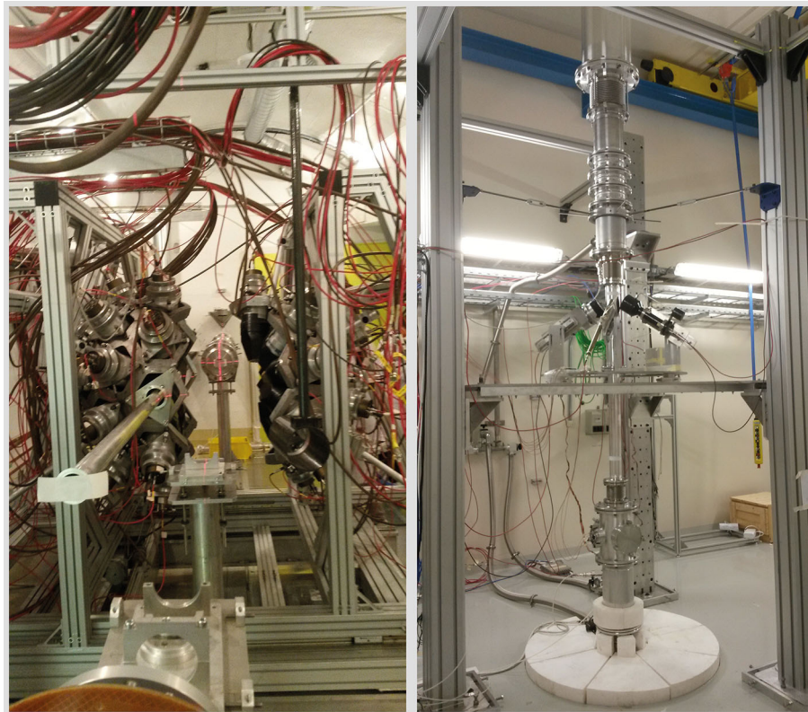
Fig. 4. Picture of the horizontal neutron beam line in EAR1 (left panel) showing the TAC in open position, and the vertical neutron beam line in the newly constructed EAR2 (right panel), showing a neutron capture setup with C_6D_6 detectors above the chamber containing the silicon neutron beam monitors (SiMon2).
