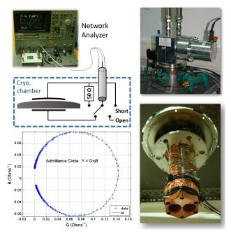
FIG. 2: Experimental set up and resulting plot after processing. Photographs show clockwise: the network analyzer; the outside part of the cryogenerator; the two stages of the cryogenerator once the vacuum enclosure removed, G(B) data plot and a fit.
