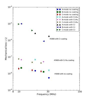
FIG. 3: Mechanical losses  $\phi=1/Q$  versus frequency of low-order OTs of the A, B and C modes, at 4 K, for sample 5808 in three different situations: uncoated substrate, Gold evaporated on both surfaces, Chromium on both surfaces.
