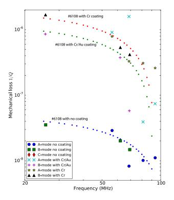
FIG. 4: Effect of gold and chromium coatings on sample 6801 in comparison with the case of the uncoated substrate, in terms of mechanical loss  $\phi=1/Q$  versus frequency, at 4 K. Higher OTs than in Fig. 3 are presented here for the A and B modes. Dotted lines are the linear regressions for the data.
