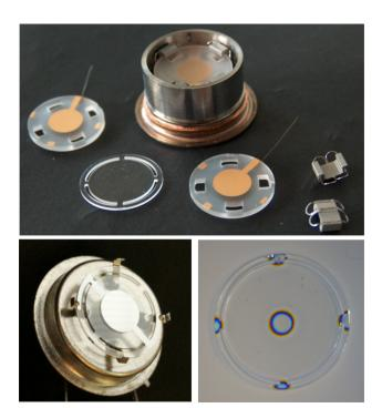
FIG. 1: Examples of devices under test. Upper photograph: an electrodeless quartz resonator (whose outer diameter is 13.2 mm). Lower left photograph: a resonator with chromium electrodes; Lower right photograph: a resonator with  ${\rm Ta_2O_5/SiO_2}$  coating.
