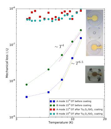
FIG. 5: Mechanical losses 1/Q versus temperature of a quartz resonator without and with a single surface silica/tantala coating. OTs of A (extensional) and B (thickness shear) modes are at 34.244 MHz and 27.280 MHz respectively. The coated resonator is shown between both electrode holders in the left inset.
