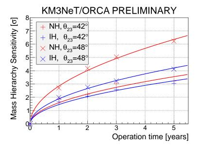
**Figure 5:** NMH sensitivity as function of data taking time with ORCA for both NMH hypotheses and two values of  $\theta_{23}$ . With the exception of the CP-phase all considered systematic uncertainties are taken into account.
