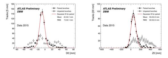
Figure 5: Radial distance (left plot) and longitudinal distance (right plot) of the closest approach of the projected particle tracks to the interaction point as recorded by a single DBM telescope with no alignment included yet.
