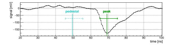
Figure 1: A sample signal trace. The horizontal bars indicate the regions where pedestal (dashed) and signal (solid) were calculated.
