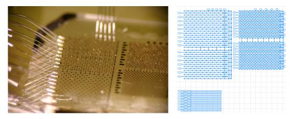
(a) Photo of the 3D device showing the metalization pattern
