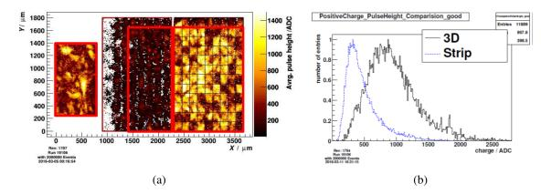
Figure 4: a) Average pulse height versus predicted hit position in the strip, 3D phantom and 3D pattern (from left to right) b) Pulse height distributions of the 3D detector in the fiducial region of (a) (marked in green) compared with the pulse height distribution of the strip detector measured with the same electronics on the same diamond.
