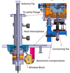
Figure 3: MINERVA spoke power coupler.
