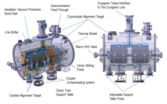
Figure 1: MINERVA spoke (beta=0.37, 352 MHz) cryomodule conceptual design.
