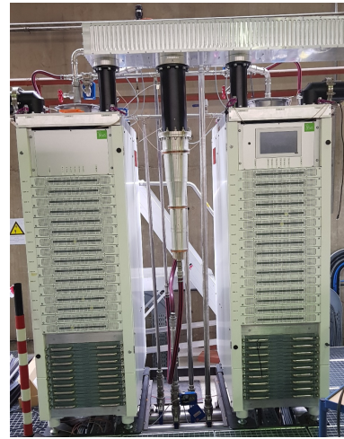
Figure 8: 192 kW Solid State Amplifier driving the MYRRHA RFQ.
