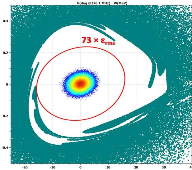
Longitudinal acceptance (white area of the plot) and considered 16.6 MeV input beam distribution.
