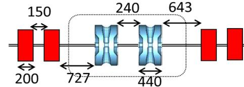
Section #2 -  $\beta \sim 0.5$  double spoke section
