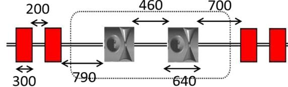
Section #3 -  $\beta \sim 0.7$  Elliptical section
