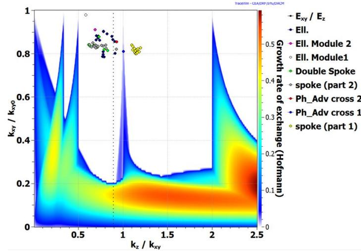
Zero-current phase advance (per meter) law and tuning set-points in the Hofmann diagram (after section matching).
