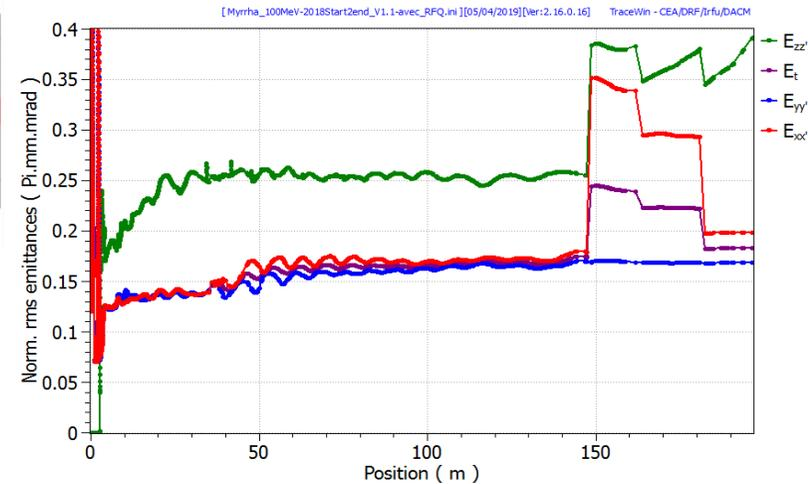
Normalized RMS emittance evolutions through the MINERVA linac
