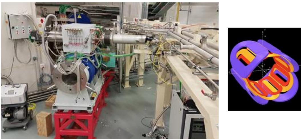
Figure 4: [Left] Photograph of a superconducting multipole triplet under cryogenic tests at Ganil. [Right] Schematics of the quadrupole (violet) sextupole (yellow) and octupole (red) coils.
