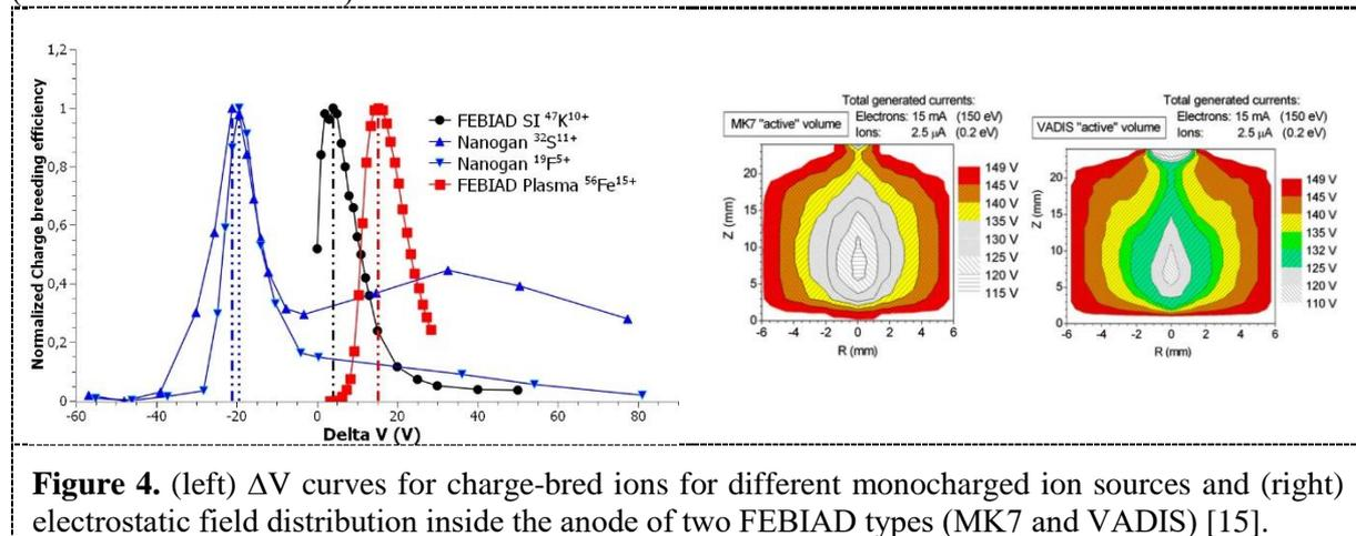
**Figure 4.** (left)  $\Delta V$  curves for charge-bred ions for different monocharged ion sources and (right) electrostatic field distribution inside the anode of two FEBIAD types (MK7 and VADIS) [15].
