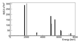
FIG. 11. Comparison between the calculated (black) and experimental (light gray)  $B(E2; 0_{g.s.}^+ \rightarrow 2^+)$  strength distribution in <sup>68</sup>Ni, up to  $S_n=7.79$  MeV (see text for explanation).
