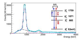
FIG. 2. (Color online) Doppler-corrected and backgroundsubtracted  $\gamma$ -ray spectrum of <sup>70</sup>Zn measured with Château de Cristal (black histogram). The intensities of the two peaks were determined using the simulated response function of the array (dashed magenta line) on top of two exponential functions accounting for the background (long-dashed gray line). The result of the best fit procedure is illustrated with blue circles.
