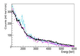
FIG. 7. (Color online) Comparison between the experimental Doppler-corrected energy spectrum for a <sup>68</sup>Ni beam on a C target (solid black histogram) and simulated spectra assuming  $\beta_N = 0.1$  (magenta stars) and  $\beta_N = 0.2$  (dashed blue histogram). The adopted value of  $\beta_N = 0.102(8)$ , as deduced from the study with the Pb target, is too small for a peak to be seen when <sup>68</sup>Ni scatters off the C target.
