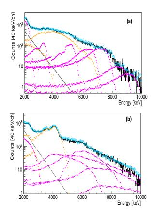
FIG. 8. (Color online) (a): Doppler-corrected experimental  $\gamma$ -ray spectra of  $^{68}$ Ni (black histogram) compared to GEANT4 simulations (open blue circles) including the excitation of several in-flight  $\gamma$ -ray components (magenta squares) discussed in the text and the excitation of the  $2^+_1$  and  $3^-_1$  states of the  $^{208}$ Pb target (orange triangles). (b): same as (a) but non Doppler-corrected.
