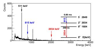
FIG. 1. (Color online)  $\gamma$ -ray spectrum of one HPGe detector associated with the de-excitation of <sup>68</sup>Ni implanted in the plastic detector. The lines corresponding to the decays of the  $0_2^+$  and 5<sup>-</sup> isomers are indicated by arrows.
