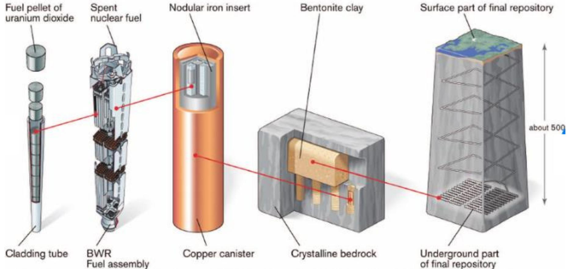
The KBS-3 method. The method involves encapsulating the spent fuel in copper canisters which are then emplaced, surrounded by a buffer of bentonite clay, in deposition holes in a tunnel system at a depth of 400 Å 700 m in the bedrock (SKB, 2011, reproduced with permission). BWR: boiling water reactor.
