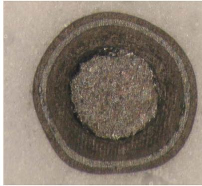
Sintered glass with pretreated particles
