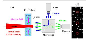
FIG. 1. (a) A schematic illustration of the experimental setup. The pink arrows indicate the electric field direction. (b) Snapshots of bead position in a time sequence of proton irradiation at 1.9 MGy s<sup>-1</sup>. The proton beam is centered in the 12  $\mu$ m diameter red circle.
