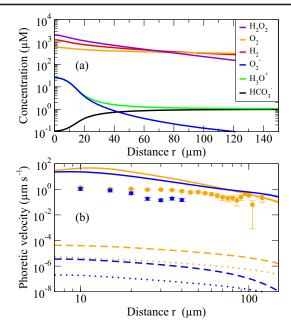
FIG. 4. (a) Concentration profiles at t=5 s. Calculations are performed with the reaction-diffusion model at a dose rate of 1.9 MGy s<sup>-1</sup>. (b) Experimental (symbol) and calculated bead migration velocities at dose rates of 30 kGy s<sup>-1</sup> (blue) and 1.9 MGy s<sup>-1</sup> (orange). Calculated velocities induced by polar neutral [Eq. (6)], apolar neutral [Eq. (7)], and charged [Eq. (8)] species gradients are reported in dashed, dotted, and solid lines, respectively.
