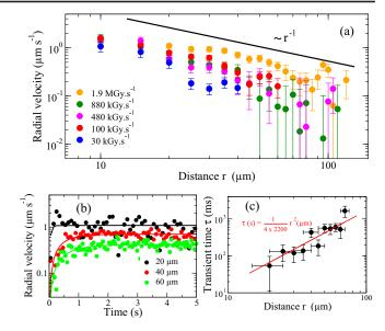
FIG. 2. (a) Steady-state radial velocity profiles measured for proton dose rates ranging from  $30\,k\text{Gy}\,\text{s}^{-1}$  to  $1.9\,\text{MGy}\,\text{s}^{-1}$ . (b) Time evolution of the radial velocity of the beads measured at three different distances from the center of the proton beam at  $1.9\,\text{MGy}\,\text{s}^{-1}$ . (c) Evolution of the characteristic time  $\tau$  of the transient state as a function of the distance from the beam axis at  $1.9\,\text{MGy}\,\text{s}^{-1}$ .
